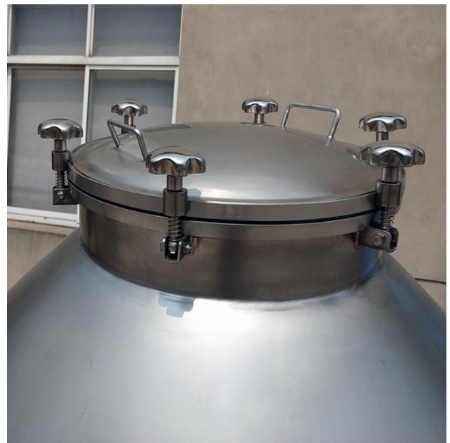
Feeding Port (Manhole) of PDC Mixer
