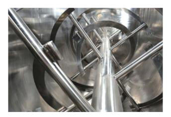
The shaft is sealed with stuffing box with multiple PTFE packings (sometimes with a lantern ring for air purge) at both ends. Materials are loaded from top side, and a flush fitting discharge valve is located at the bottom side in the center. The discharge height can be adjusted as per requirement, so that material gets discharged into the container below it without floating dust.
