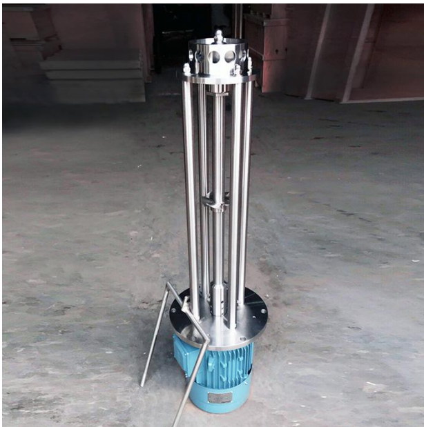
PS-D Mixer with Lifting Hanger
