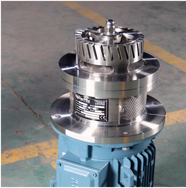
PS-B Bottom Mounted Mixer
