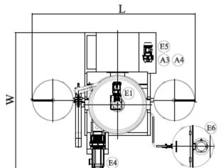
A: Water connection E: Electrical connection D: Drain port
