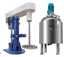
PerMix PD High Speed Disperser works with the powerful high speed rotation of the saw disc impeller. Liquid or solid materials are subject to the high shear force at the periphery of the saw disc when the impeller is rotating at high speed, and they are dispersed quickly and efficiently into the liquid body, after short time, homogeneous dispersion is produced.
