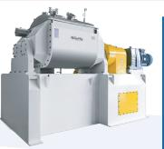
With its unique design of Z-shaped mixing tools installed in two semi-cylinders, the PerMix PSG series Sigma Mixer is able to provide a combined functions of compressing, stretching, folding, kneading & mixing, which makes it widely used in the chemical, food, sealing compound and paint industries, among others. If a screw extruder is applied for discharging, the mixer is also called Sigma Mixer Extruder, or Mixtruder.
