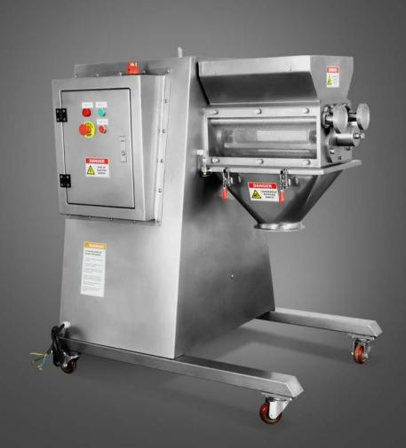
PerMix POG Oscillating Granulator is designed to process wet powder and block dry powder materials into fine and consistent granules. By working with meshes of different sizes, it can produce granules with various desired particle sizes.
