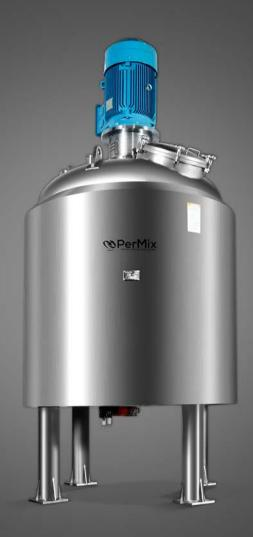
The PerMix PD series High Speed Disperser (or Dissolver) is ideally designed to meet the demands of a broad spectrum of industrial applications for dispersing purpose of solid or liquid materials into liquid body.
