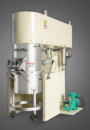
The PerMix PDP series Double Planetary Mixer is also called double planetary kneader, because it can be used to handle very viscous materials up to 1,500,000 cPs. Usually the PerMix PDP series Double Planetary Mixer has two vertically mounted mixing tools which are driven by one gear to move around the central axe of the tank as well as their own axis.
