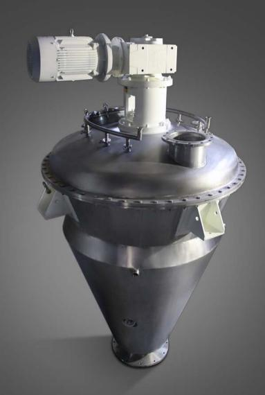
The PerMix PVR series Vertical Ribbon Mixer has a similar appearance with the PRB series Ribbon Blender, but stands vertically, same as our PNA series Conical Screw Mixer. PVR Vertical Ribbon Mixers are efficient and versatile blending machines for batch mixing of free-flowing powders, granules and pellets.
