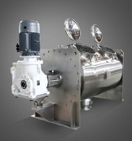
The PerMix PTP-D series Vacuum Mixer Dryer is a turbulent mixing reactor-dryer. It is used as a high-speed mixer dryer, chemical reactor or, if both processes are combined, as a dryer-reactor. They are used with particular success in agglomeration-free rapid drying, heterogeneous reactions with systems of different substances, extraction, sterilization and in general for vacuum, positive-pressure, thermal energy and comminuting aids.
