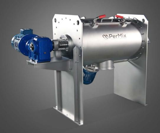
PerMix PTS series Plow Mixer is one of our two types of Turbulent Mixer, which are originally designed by our Israeli engineers. The other one is PTP series Paddle Mixer.
