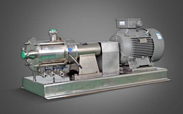
An inline mixer is a high shear mixer for inline or continuous operation. In the Inline process, the mixer is installed outside the tank. This makes it easy to be built into an existing production line with normal inlet/outlet connections.
