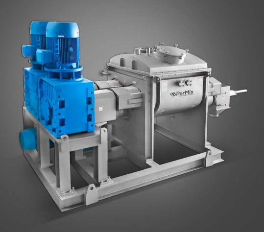
PerMix PSG-X Sigma Mixer Extruder (or Mixtruder) is designed with an extrusion screw located in a cylindrical barrel in the middle and below the two mixing arms. The extrusion screw is used to discharge the product, but can also runs in reversed direction during mixing cycle, lifting materials up to the reach of mixing arms, thus assuring a thorough kneading and accelerating the mixing process. The screw has its own separate drive.
