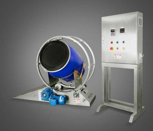
The PerMix PDR series Drum Hoop Mixer has been developed to meet increasing demands for a low batch mixer for mixing, blending, homogenizing, dyeing of dry powders and granules particularly in smaller industries or when frequent product changes as required.
