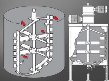
PerMix PCR series Contra Rotating Mixers are typically used when thick emulsions are produced by a bottom entry high shear emulsifier or homogenizer.
