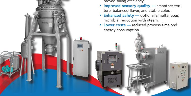
From a technical standpoint, instantization is a controlled balance between heat, moisture, and motion — and PerMix has perfected that balance. By merging fluidized mixing with steam or atomized liquid dosing, the PerMix system creates powders that are safe, stable, and instantly functional.
